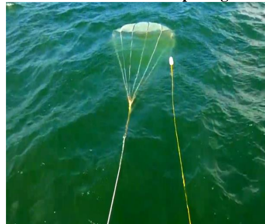
4. Deployment of sea anchor
