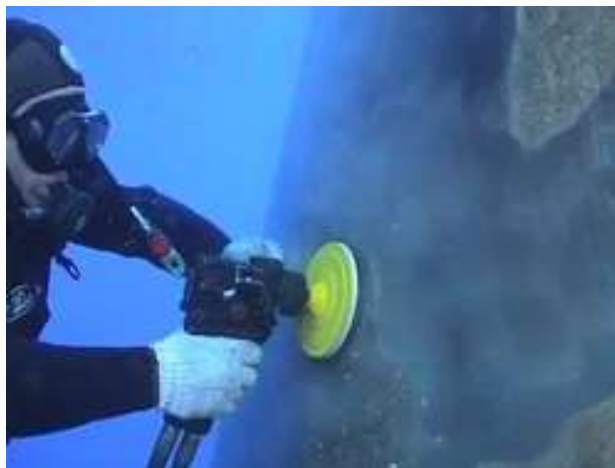
Figure: Rotary Brush hull Cleaning
