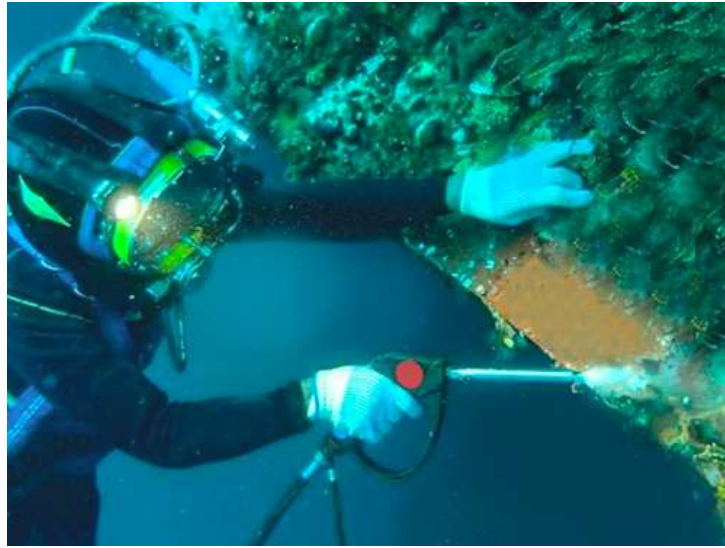
Figure: Cavitating Water Cleaning Jets
