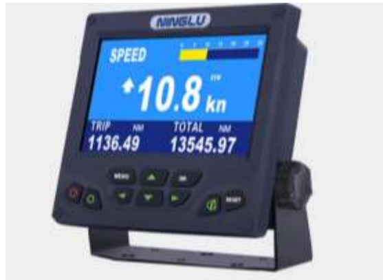
Figure 5. Speed and distance log device
