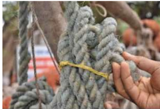
Rope made from Nylon monofilament gillnets
