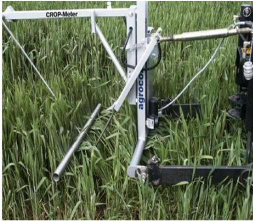
Fig. Crop biomass sensor in the Field Fig. working principle of sensor for crop biomass Measurement
