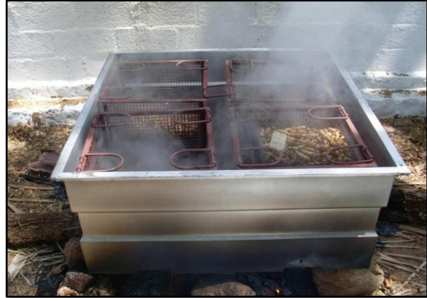
Steam boiling of turmeric in TNAU designed boiler
