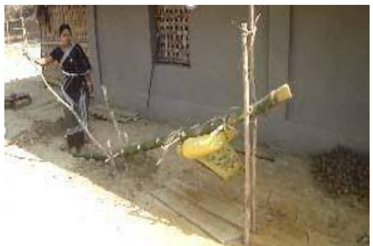
Paddle-operated polishing method
