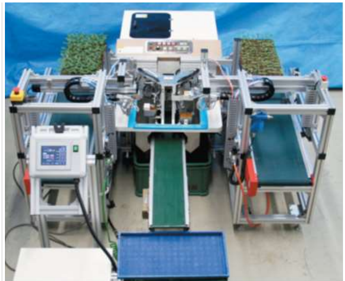
Fig. 2 Fully automated grafting robot for cucurbits (BRAIN, Saitama, Japan)
