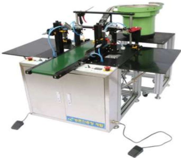
Fig. 1 Semi-automatic grafting robot
