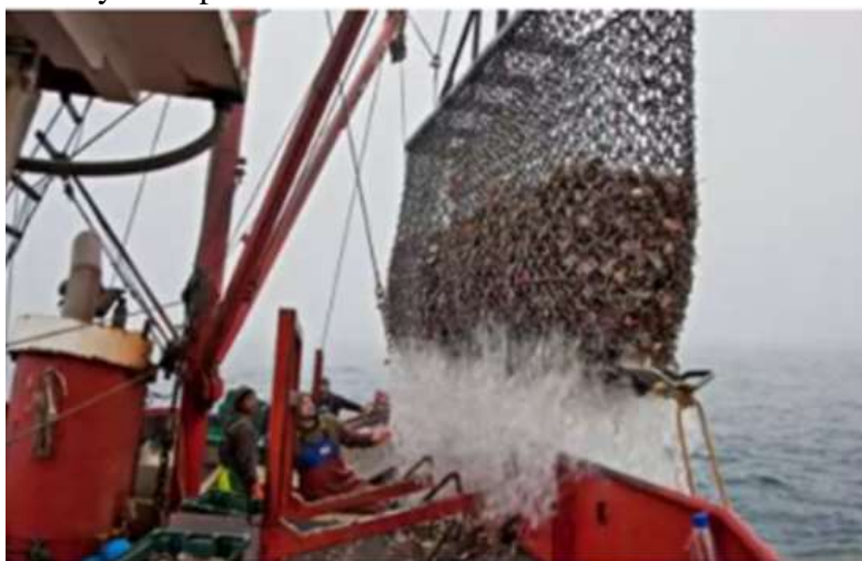
Figure 6 Rigid Dredge in operation
